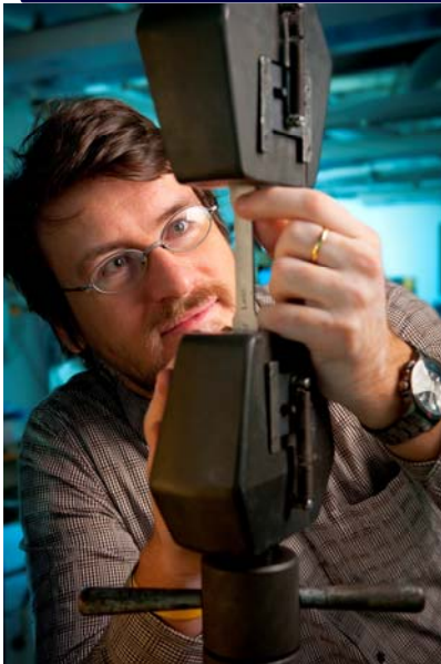
Professor Korkolis preparing a uniaxial tension test. Photo Courtesy Perry Smith
